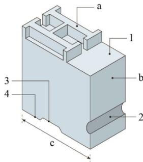
Figure 1. Type structure: a – face, b – body or shank, c – point size; 1 – shoulder, 2 – nick, 3 – groove, 4 – feet
